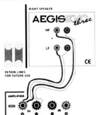
BI-WIRING [OR MULTI WIRE] CONNECTION
